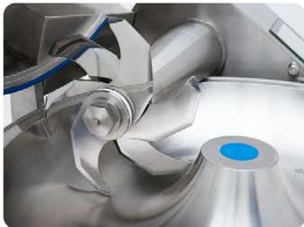
Removable 6-knife head and compensating rings for use with 3.
