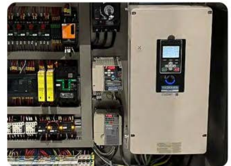
Soft start and stop of knives, bowl and extracting disc (optional) by mean of speed drives.
