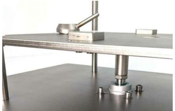
CE approved gaps on all moving parts, no trap points on machine.
