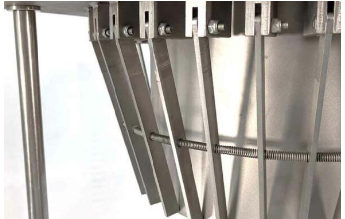
Spring loaded fingers, no adjustment required for different tubes.
