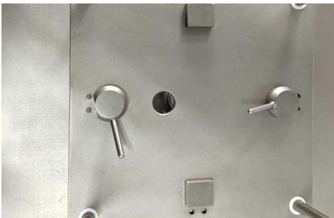
Quick release cam lock without tooling.
