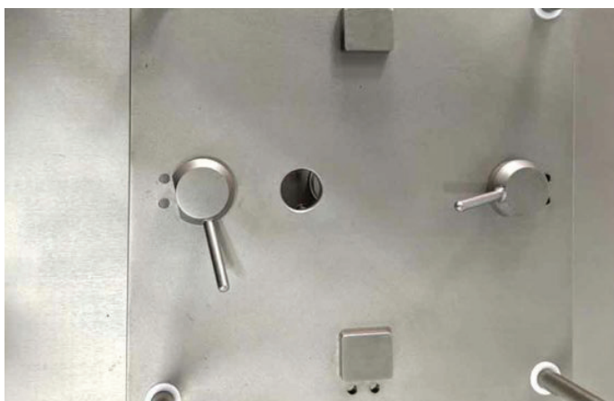
Quick release cam lock without tooling.
