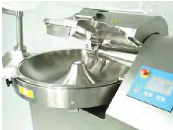
Stainless steel motorized knife lid for effortless lifting and lowering.
