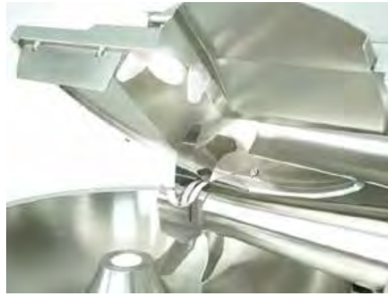
Smooth polished surfaces, no corners or screws, with \text{C}\epsilon radius for easy cleaning.
