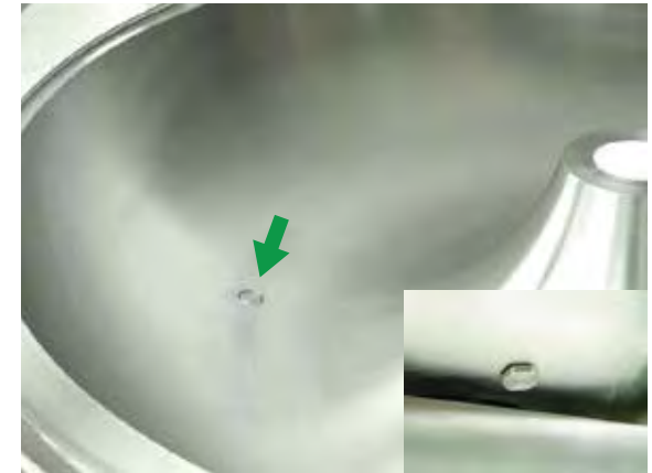
Bowl with drain plug with automatic positioning.
