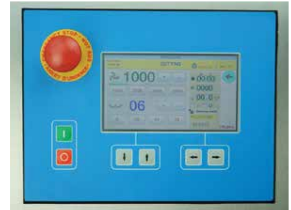
Digital display to control and program all functionalities of the cutter.
