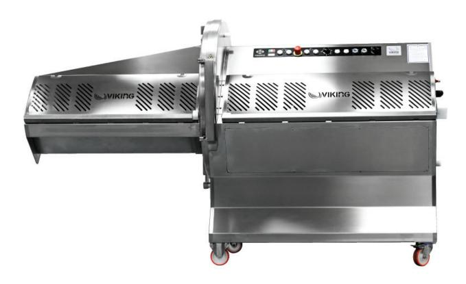
For slicing fresh, frozen and cooked products like beef, veal, pork loins and other bone-in and boneless products like cheese in equal thickness. Cutting thickness can be adjusted also during operation from 1 to approximately 40 mm. Slicing mode can be selected. The product advances step by step with normal mode or continuously for extra thin slicing mode.
