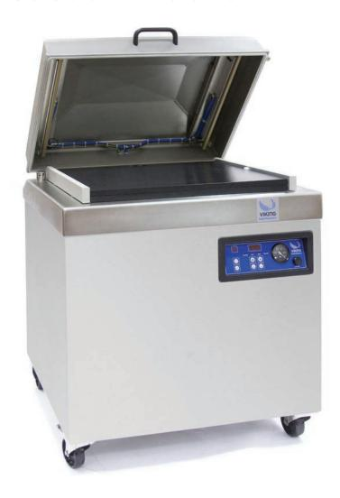
Easy to operate and clean, the V423 model with its flat Stainless Steel working plate and double seal bars has increased capacity for packaging large and specialised products such as cheese wheels and full leg hams.
